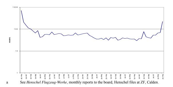
Figure 8 Labor costs per Ju 88 wing set, planned in advance and actually needed, Siebel 1942<sup>a</sup>
